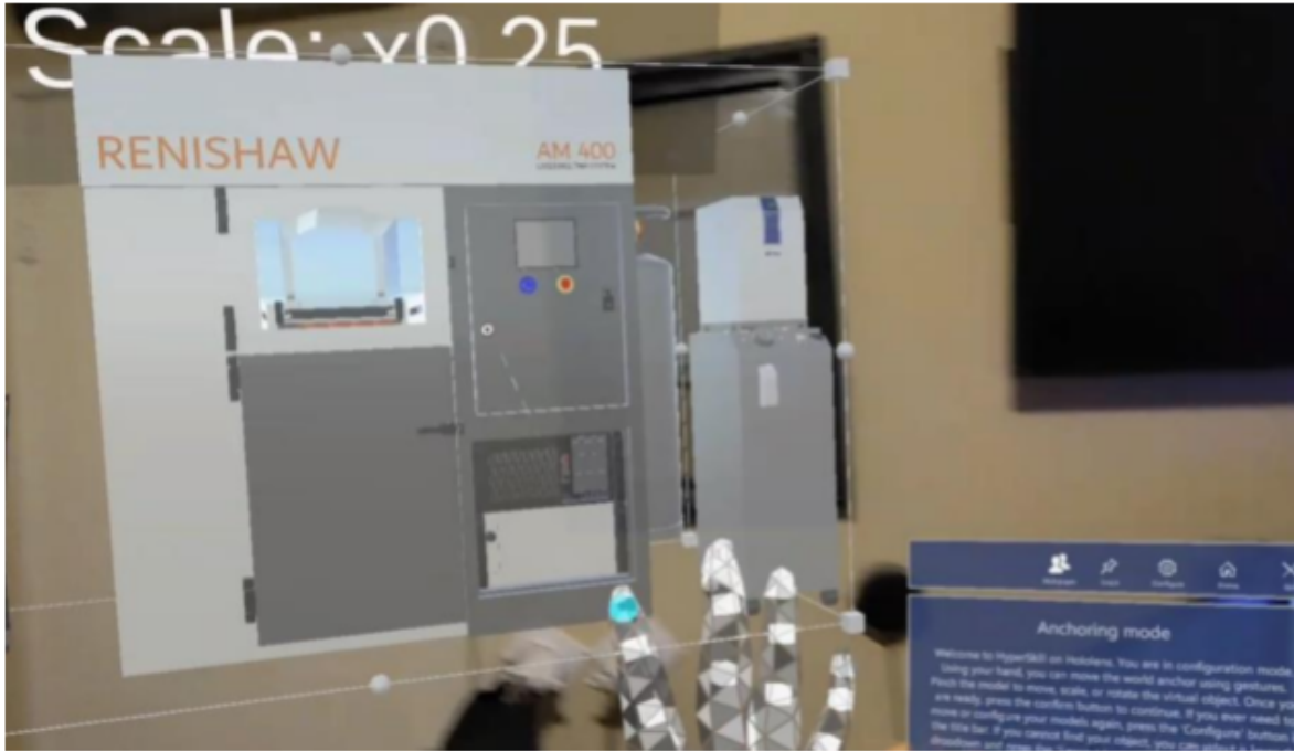
Figure 3: AR visualization of the Renishaw AM400
