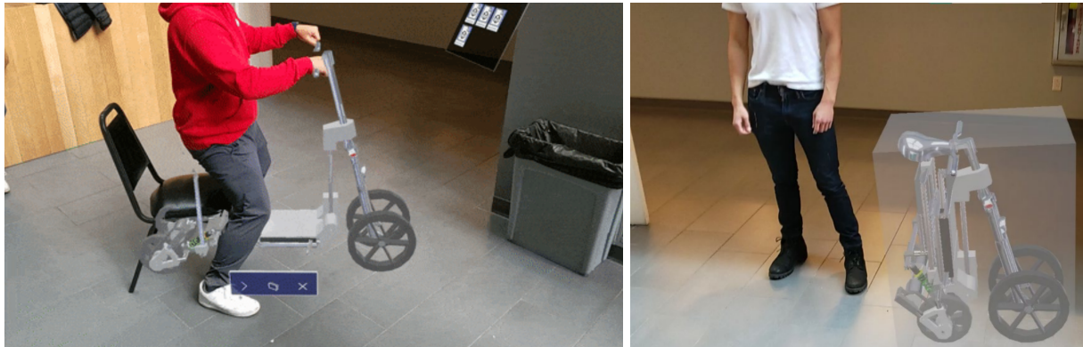
Figure 3: Students visualizing models in different states and verifying scale and fit. Visualizing life size holograms of designs prior to ordering components and starting fabrication of prototype 2
